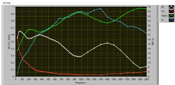
Absorption coef. (green line), Reflection coef. (white line), Transmission coef. (red line), Transmission Loss (blue line).
