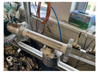
Hollow Silent pipe (L: 60cm D: 16cm) with Low transmission coef. and high absorption.
